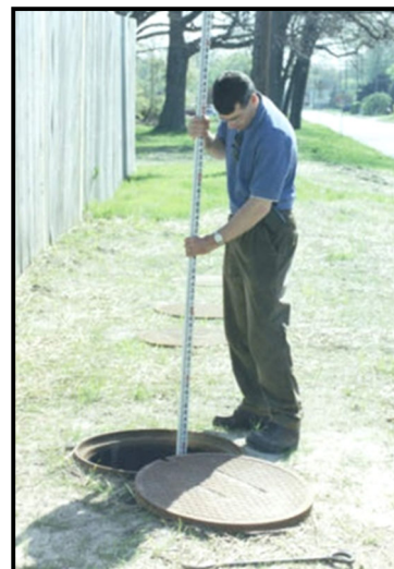
Sediment inspection using a stadia rod
