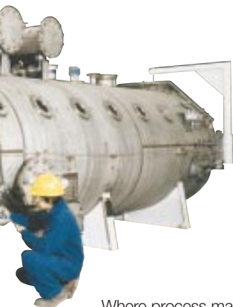
Where process material or fumes are hazardous, the filter can be fitted with a totally vapor-tight enclosure. Vapors are condensed from the process gas before the gas is returned to the enclosure. This machine replaced centrifuges, increasing throughput and product quality.
